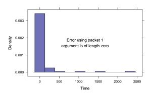
It appears that the distribution of Time is highly skewed with a long right tail. Therefore one possible transformation would be to take the log of the Time observations.
